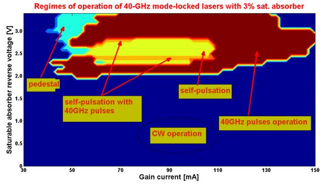
Fig. 2. Experimental operating regime map as a function of the bias current applied to the gain section (horizontal axis) and the reverse voltage applied to the SA section (vertical axis). Blue, light blue, yellow and red indicate no ML, incomplete ML, ML with SP and stable ML, respectively.
