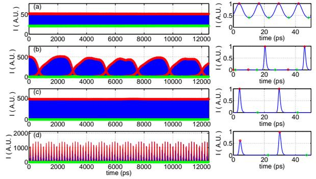
Fig. 1. Long time behavior of the time traces of the field intensity (left) and details of the pulse shape (right). The panels a), b), c) and d) correspond to  $l = 1.5\%$ ,  $l = 3\%$ ,  $l = 3.75\%$  and  $l = 6.5\%$ , respectively
