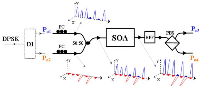
Figure 1. SOA balanced-receiver. Insets shows RZ-DPSK case.
