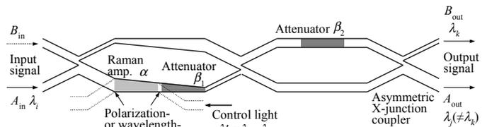
Figure 2 Schematic diagram of the modified switch.
