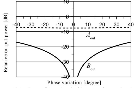
(a) At the condition when incident wave is routed to  $A_{out}$
