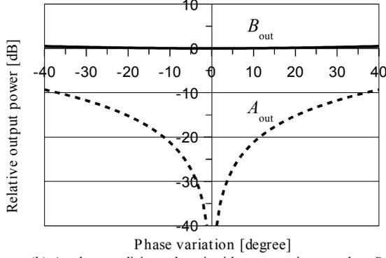
(b) At the condition when incident wave is routed to  $B_{out}$
