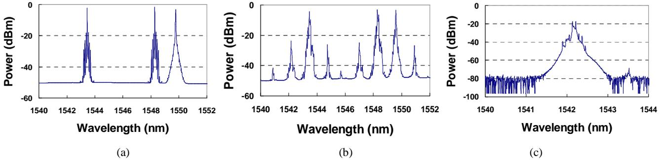
Fig. 2 Measured optical spectra (a) before SOA (b) after SOA (c) one converted RZ signal
