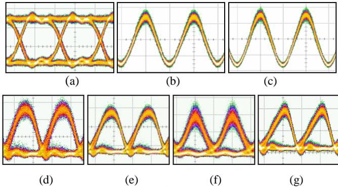
Fig. 3 Measured eye diagrams before and after the conversions (Time scale: 50 ps/div)
