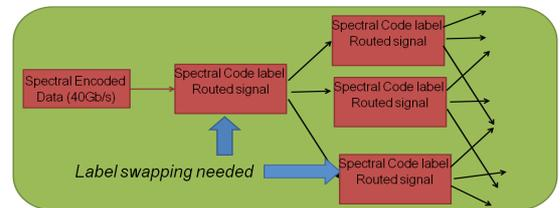
Fig.1. Multi-hop spectral coded label self switched network
