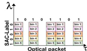
Fig.2. Optical packet format
