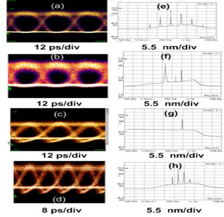
Fig. 4. (a) Original eye diagram of the 40 Gb/s Code 20 spectrally encoded data; (b) 40 Gb/s encoded signal after self routing by FWM; (c) 40 Gb/s encoded signal after wavelength conversion by XGM; (d) 40 Gb/s encoded signal with Code 19 after self routed by FWM; (e) Spectrum of Code 20 after FWM in the forwarding node; (f) spectrum of filtered 40 Gb/s signal and the CW used in the XGM process; (g) converted 40Gb/s data (h) 40Gb/s coded signals after FWM at the receiver.
