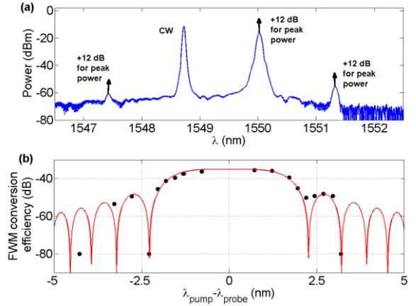
Figure 2. (a) FWM optical spectrum for a CW probe and a modulated pump. (b) FWM efficiency dependence on pump probe detuning for the pump wavelength of  $\lambda_p = 1550$  nm (dots). The solid line represents a simulation.
