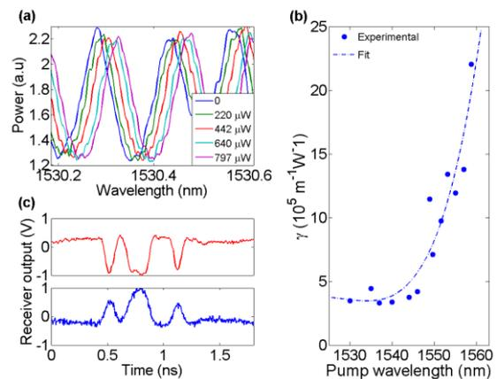
Figure 1. (a) Fabry Perot fringes as a function of wavelength for various input pump powers. (b)  $\gamma$  values as a function of pump wavelength (dots). (c) Pump (red trace) and probe (blue trace) dynamics for a 10 Gbit/s pattern.
