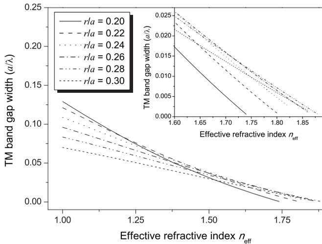
Figure 2. TM band gap width as a function of effective refractive index of the mode in vertical waveguide layer stack and normalized pillar radius  $r/a$  for 2D pillar photonic crystals.  $r$  denotes pillar radius,  $a$ , photonic crystal lattice constant,  $\lambda$ , wavelength.
