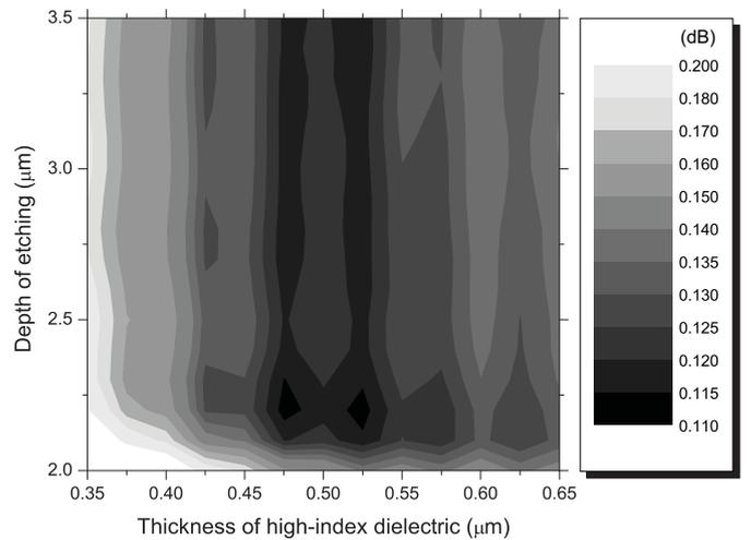
Figure 3. Coupling loss on advance through an interface of 2D pillar photonic crystal as a function of thickness of high refractive index material and depth of etching. Plot is limited by thickness of high refractive index material = 0.65  $\mu\text{m}$  since larger values cause closure of photonic band gap.
