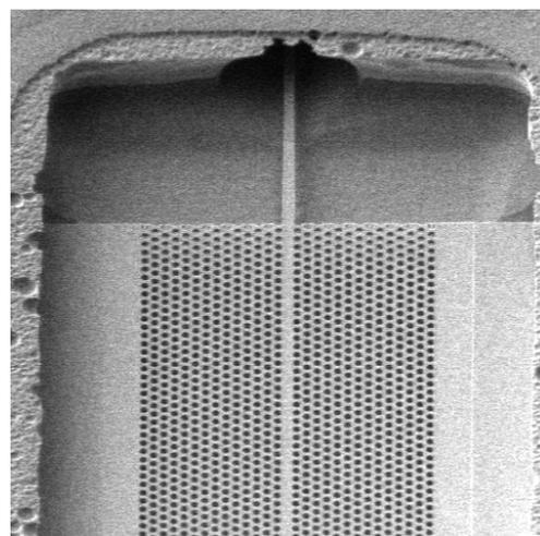
Fig. 1 Si PCW integrated with photonic wire by using CMOS technology
