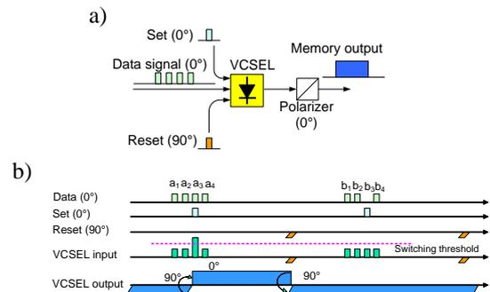
Figure 2. 1-bit buffering using a PB-VCSEL. a) Implementation and b) Timing chart.
