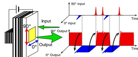
Figure 1. Polarization bistable operation by injection of optical pulses in a VCSEL.
