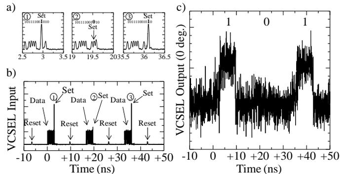
Figure 3. Memory operation for 20-Gb/s,  $2^6$ -1 bit PRBS RZ signals. a) Magnified VCSEL input, b) VCSEL input, and c) VCSEL output.
