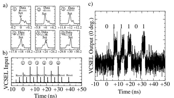
Figure 4. Memory operation for 40-Gb/s, 6-bit NRZ signals. a) Magnified VCSEL input, b) VCSEL input, and c) VCSEL output.
