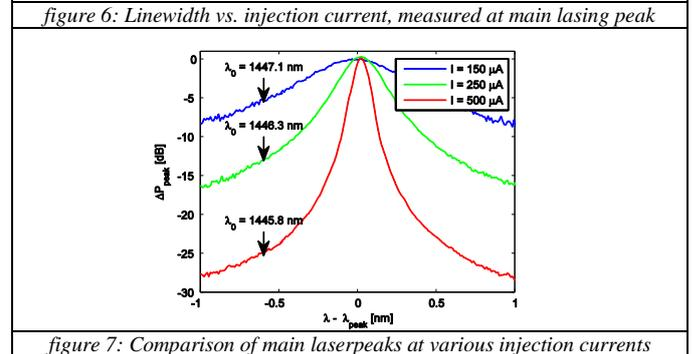
The wavelength of the peaks is 1447.1 nm, 1446.3 nm and 1445.8 nm respectively. The smallest linewidth measured for these devices is 68 pm, but is possibly smaller due to the limited resolution of the spectrum analyzer. The Fabry-Perot cavity modes are spaced 3 nm apart, which corresponds to a FSR = 444 GHz.
