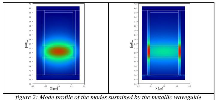
figure 2: Mode profile of the modes sustained by the metallic waveguide
