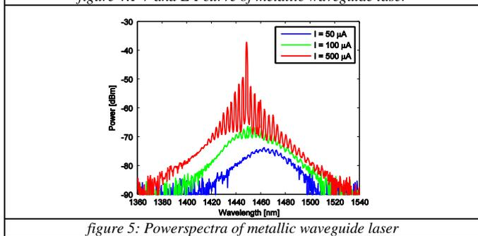
The wavelength of the main laser peak is located close to 1450 nm. The considerable blue shift is due to the high current density inside the device, the high gain required for lasing and the low operating temperature. The output power level at the wavelength peak 0.14  $\mu\text{W}$  (in-fiber).
