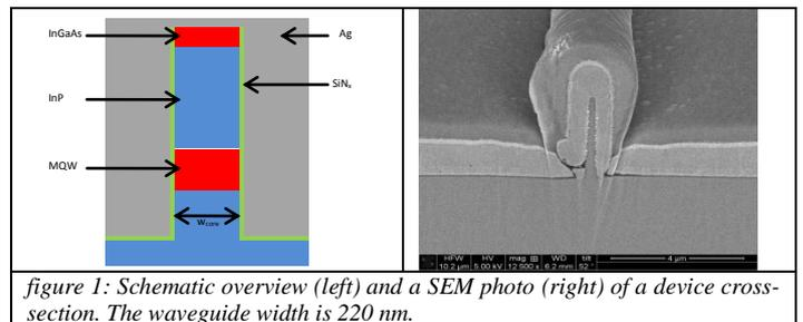
figure 1: Schematic overview (left) and a SEM photo (right) of a device cross-section. The waveguide width is 220 nm.
