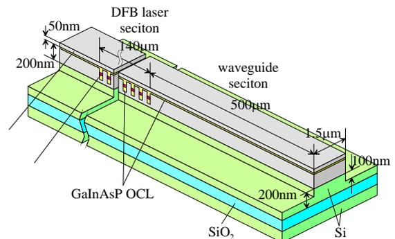
Fig. 2 Schematic of membrane BH-DFB laser directly bonded on SOI with rib-waveguide [30].
