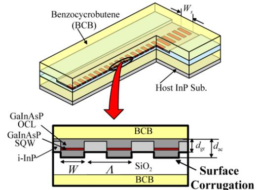
Fig. 1 Schematic of membrane BH-DFB laser with surface corrugations [27].
