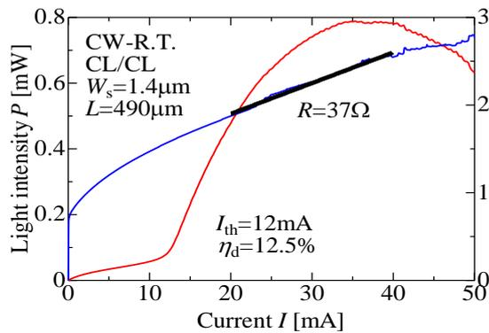
Fig. 3 Light output and voltage-current characteristics of LCI-BH laser grown on SI-InP substrate [33].
