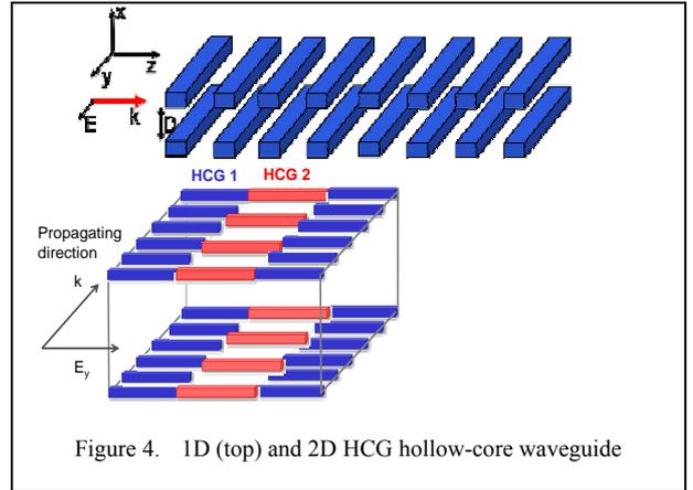
Figure 4. 1D (top) and 2D HCG hollow-core waveguide
