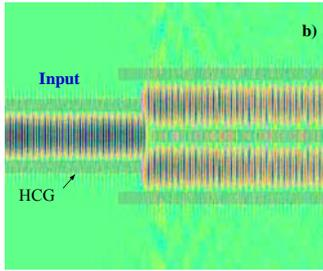
Figure 5. Finite-difference time domain simulation showing the splitting of light in a HCG-HW based MMI splitter.
