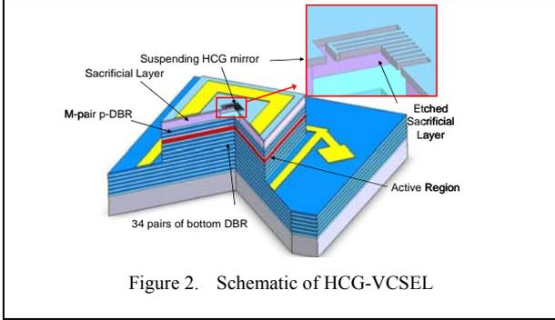
Figure 2. Schematic of HCG-VCSEL
