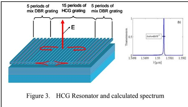
Figure 3. HCG Resonator and calculated spectrum
