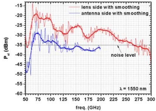
Figure 5. Frequency response of micro-pin antenna chip.
