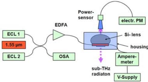
Figure 3. Heterodyne based measurement setup.
