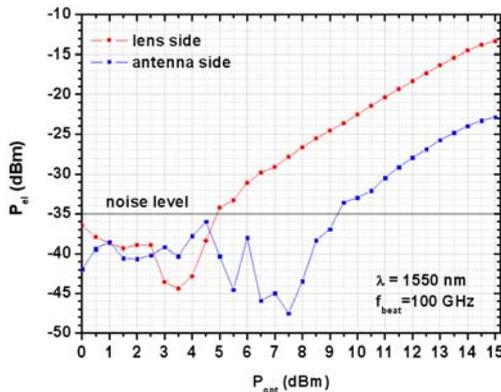
Figure 4. Output power vs. optical input power.
