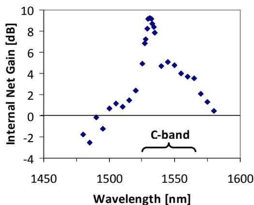
Figure 1. Internal net gain in an Al<sub>2</sub>O<sub>3</sub> channel waveguide amplifier with an Er<sup>3+</sup> concentration of 1.17×10<sup>20</sup> cm<sup>-3</sup> as a function of wavelength
