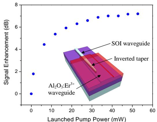
Figure 3. Signal enhancement (dB) vs. launched pump power in an  $\text{Al}_2\text{O}_3:\text{Er}^{3+}$ -Si- $\text{Al}_2\text{O}_3:\text{Er}^{3+}$  structure
