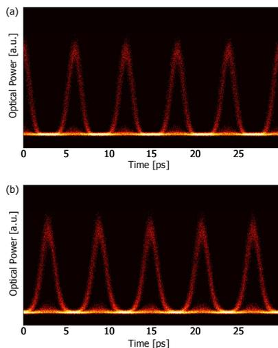
Figure 2. Transmission eye diagrams at 170 Gbit/s (a) without EDWA and (b) with EDWA and a launched signal power of 0.5 mW and counter-propagating pump power of 65 mW
