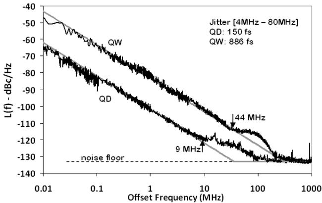
Figure 1. SSB phase noise power spectral density of the mode-locked lasers
