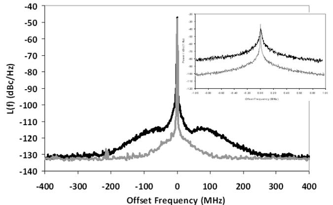
Figure 2. RF electrical spectrum showing the phase noise relative to the 10GHz carrier for the QW (black) and the QD (gray). The inset has a span of 1 MHz, and a RBW of 10 KHz
