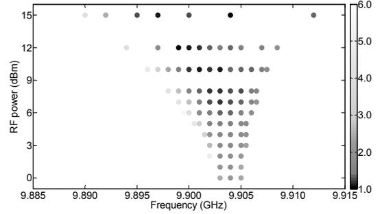
Fig.3. Time jitter (grey scaled in ps) for hybridly mode-locked QD MLLD over a range of applied RF power levels and frequencies.
