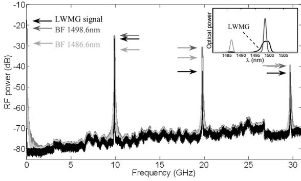
Fig.2. RF spectra obtained at  $I_{SOA}=260\text{mA}$ ,  $V_{SA}=-0.5\text{V}$ , recorded with resolution bandwidth of 3MHz. The arrows on the plot point to the top of RF peaks. The inset shows optical spectra of the signals.
