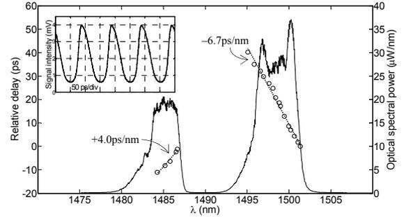
Fig.4. Relative time delay of pulses with different spectral components superimposed on a plot of the optical spectrum. The inset shows an oscilloscope trace for the LNW signal at  $I_{SOA}=290\text{mA}$ ,  $V_{SA}=-0.5\text{V}$ , and  $P_{RF}=3\text{dB}$ .
