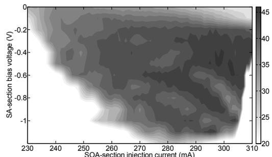
Fig.1. Height of the peak (grey scaled in dB) at the fundamental frequency over noise floor, recorded by the electrical spectrum analyzer. The electrical bandwidth used to obtain the spectra is 50kHz.
