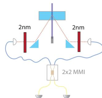
Figure 2. An SPDC two photon source with 2x2 MMI waveguide
