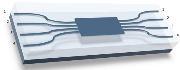
Figure 1. A 4x4 multimode interferometer, silica on silicon waveguide.
