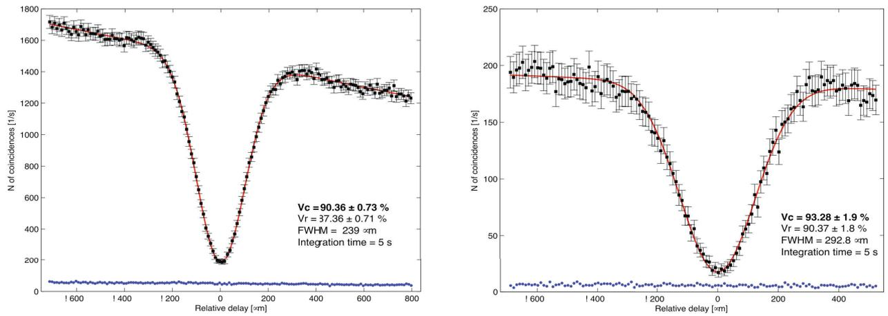
Figure 3. Quantum interference in a 2x2 MMI quantified by Hong Ou Mandel Dips. The two dips are from the same experimental set up, with the only difference being that the one on the right received post-filtering with a 0.5nm bandwidth interference filter inserted between the chip and the detector.
