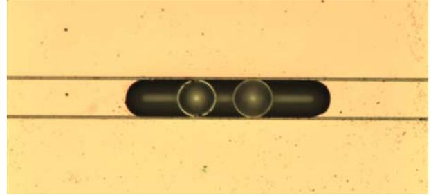
Figure 4. 60 micron microspheres assembled between waveguides
