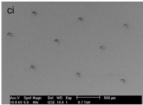
Figure 2. Glass microspheres assembled in pit array [10]
