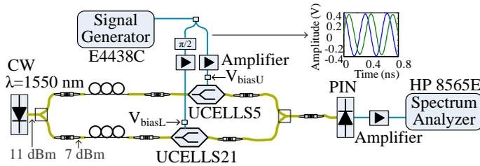
Figure 2. Experimental setup for dual-parallel Y-coupled linearized characterization
