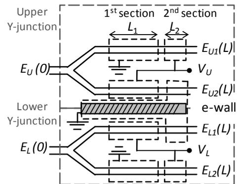
Figure 1. Proposed dual-parallel Y-coupled device structure with e-wall
