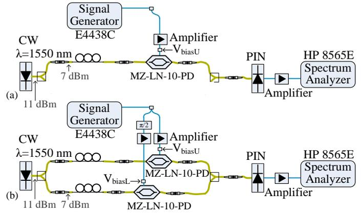
Figure 4. Experimental setup (a) single and (b) dual-parallel architecture with conventional Mach-Zehnder modulators
