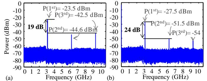
Figure 5. Measured electrical spectrum for (a) single and (b) dual-parallel architecture with conventional Mach-Zehnder modulators
