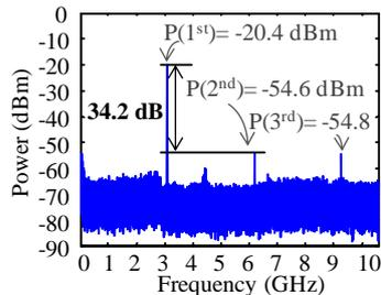
Figure 3. Measured electrical spectrum for dual-parallel Y-coupled linearized proposed architecture
