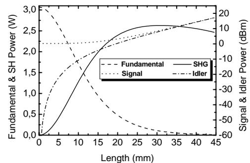
Fig. 2: Calculated evolution of cw-fundamental-, SH-, signal-, and idler power levels along the waveguide for 3 W of coupled fundamental power.
