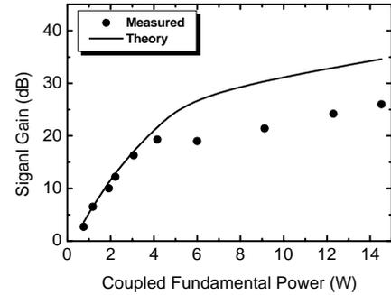
Fig. 5: Measured and calculated signal gain versus coupled fundamental peak power in a Ti:PPLN channel waveguide of 45 mm long effective interaction length and 16.3  $\mu\text{m}$  micro-domain period, operated at 165°C.
