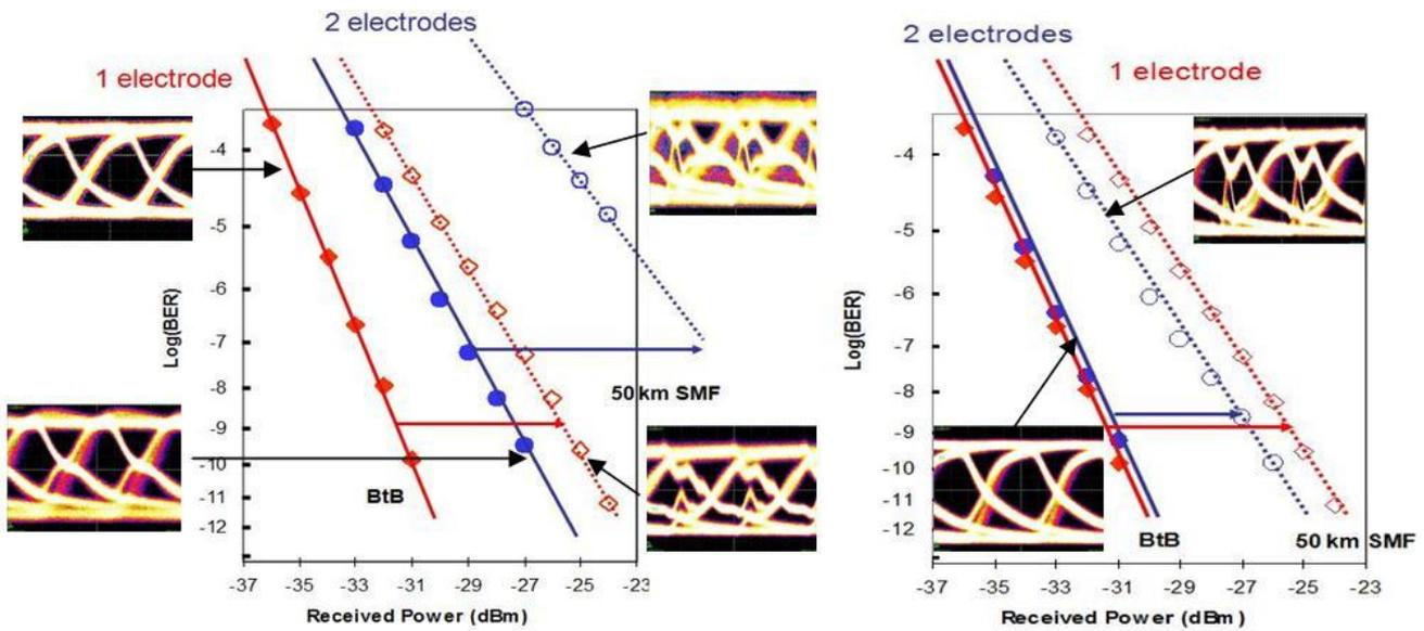
Figure 2. BER curves as a function of the received power in Back-to-Back and after 50 Km transmission for one and two electrodes configurations. In bi-electrode configuration, the modulation  $I_{HF}$  is applied to the mirror section and DC current  $I_{DC}$  to the input section (left) or inversely (right)
