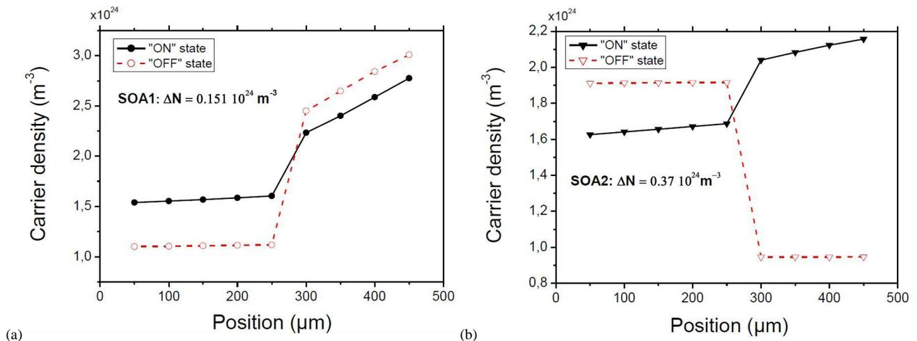
Figure 1. Simulated carrier density along bi-electrode RSOA with input (a) and mirror (b) electrode modulation for "ON" and "OFF" state
