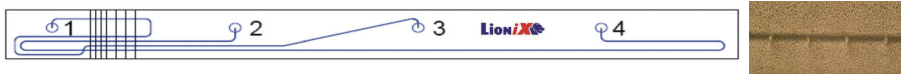
Fig. 1 Left: CE chip with integrated WGs crossing the microfluidic channels Right: Side view image of WG array – microfluidic channel intersection
