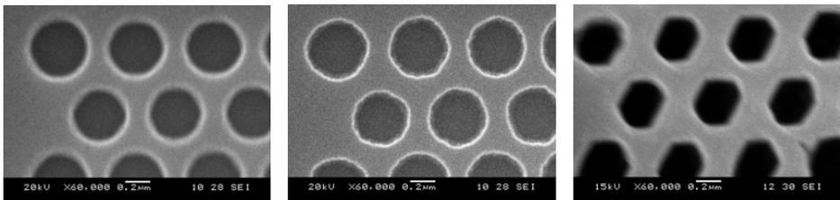
Fig. 4: Holes of a photonic crystal structure defined in photo resist (left), transferred by wet etching in the Cr film (middle) and by ICP-etching into the LN substrate.
