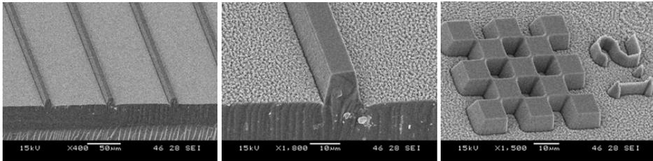
Fig. 3: ICP-etched ridges on X-cut LN of 5.8  $\mu m$  height and 8  $\mu m$  width (left and middle). Further microstructures of the same height with nearly vertical side walls (right).
