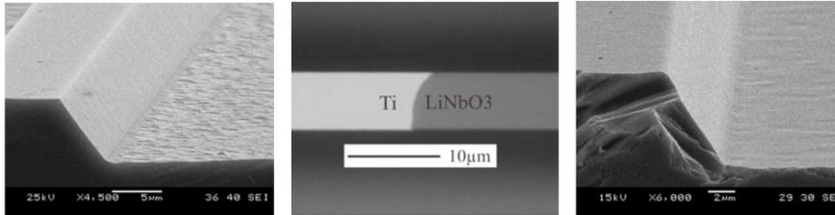
Fig. 1: Wet etched ridge on Z-cut LN, (left), Ti-coated ridge before indiffusion (middle), and after indiffusion (right). The height (top width) of the ridge is 6.5 μm (10 μm), aligned parallel X.
