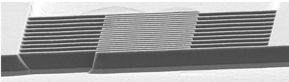
Fig. 2: Wet etched interdigital lamellas of 2.6 μm width and of 2.8 μm separation on Z-cut LN. The etching depth is 7.7 μm.
