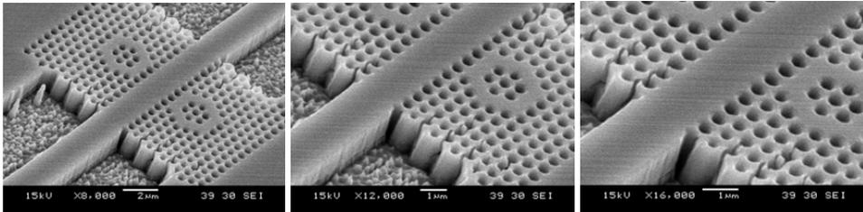
Fig. 5: Photonic crystal structure in PE-LN as a whole (left) and with more details in higher magnification (middle and right).
