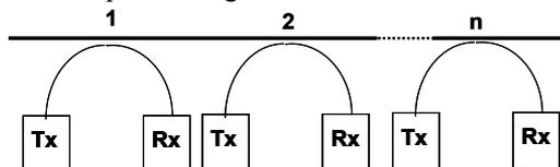
Fig.1 Optical bus architecture with passive add/drop devices.
