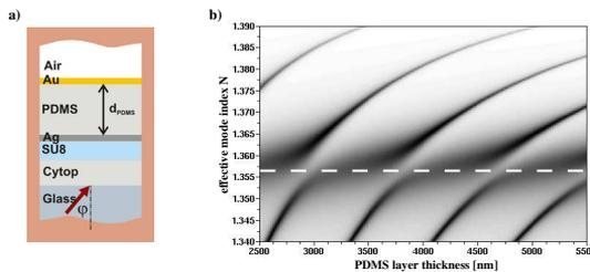
Fig. 2: Sketch of the layer system (a).  $\phi$  is the angle of light incidence. Gray scale plot of the calculated reflectance against PDMS-thickness and effective mode index  $N$  (b).
