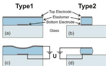
Fig. 4: Scheme of the two different geometries for time response measurements. (c) and (d) sketch the deformation which is induced by an applied voltage.
