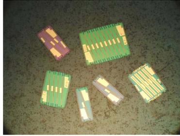
*Figure 3: Photograph of monolithic SOA chips (single, twin, quad and octo).*
