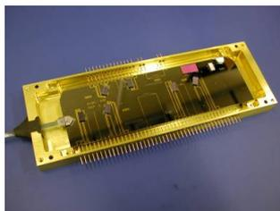
Figure 7: Photograph of the fabricated 40Gb/s BMR circuit.
