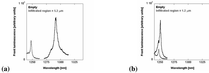
FIG. 2. Front luminescence spectra of the locally infiltrated L3 cavities shown in figure 1 (solid lines). The diameter of the polymer-filled region is (a)  $5.2 \mu\text{m}$  and (b)  $1.2 \mu\text{m}$ , respectively. The resonance peaks for the corresponding empty cavities are shown as reference (dashed lines).
