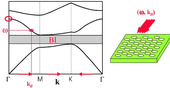
**Fig.3.** Illustration of the resonant coupling between a waveguided mode and a radiated mode.
