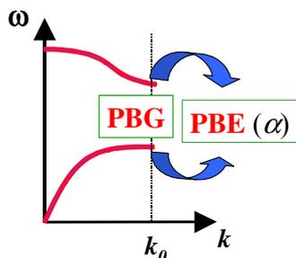
**Figure 1** : schematic representation of a photonic band gap (PBG) and of related photonic band edges (PBE) in the dispersion characteristics of a photonic crystal.
