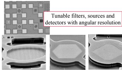
**Fig.7.** New class of MOEMS devices: structures including several InP membranes suspended in air, with a 1D and 2D PC formed in the top membrane (SEM view).
