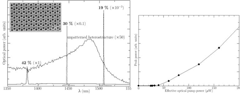
**Fig.4.** Emission spectra of the surface emitting laser formed in a graphite lattice 2D PC, for different hole filling factors ( $f$ ). The plot of the emitted power versus the pumping power indicates a threshold power of  $40 \mu\text{W}$  for  $f = 19\%$ .
