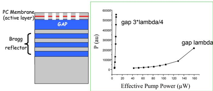
Fig.6. 2.5D Photonic Crystal micro-laser: the thickness of the top silica “gap” layer has a wide impact on the threshold power of the micro-laser
