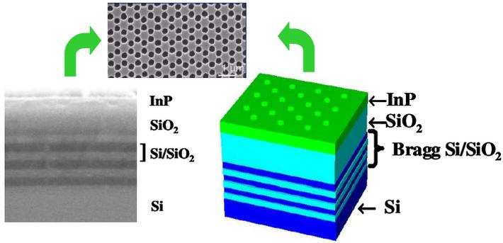
Fig.5. Photonic Crystal membrane bonded on top of a Bragg
