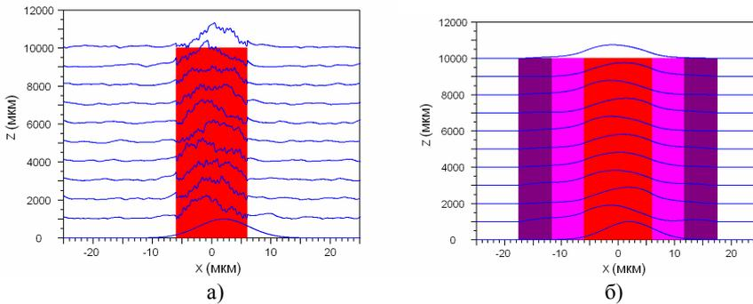
Fig. 2. Propagation of the Gaussian optical beam that is displaced by  $2 \mu\text{m}$  in relation to the axis of wide SOI waveguide. Spatial distribution of a magnetic field of TM polarization (that corresponds to TE in 3D case): a) in standard multi-mode waveguide ( $W=12 \mu\text{m}$ ); b) in heterogeneous quasi-single-mode waveguide ( $W = 12 \mu\text{m}$ ,  $W_0 = 35 \mu\text{m}$ ). 2D BPM simulation.
