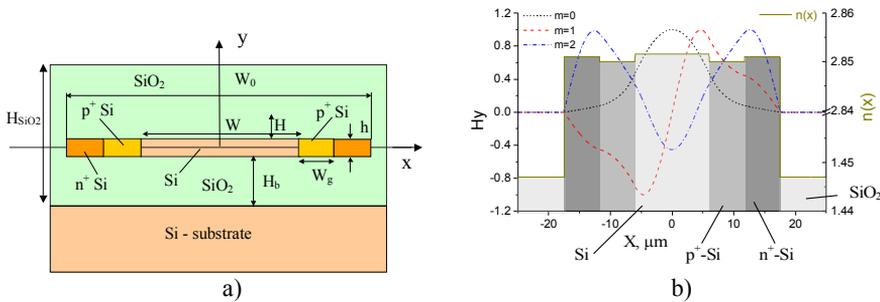
Fig. 1. Heterogeneous optical waveguide in SOI structure. a) the structure design; b) distribution of the real part of a refractive index and optical fields of the first three modes ( $W=10 \mu\text{m}$ ,  $W_0=35 \mu\text{m}$ ,  $\Delta n = 0.002$ ); Calculation by 2D BPM.
