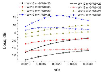
Fig. 3. Additional optical losses by free charge carriers (holes and electrons) in a strip optical waveguide for various modes as a function of real part of refractive index increment in  $p^+$ -doped regions.  $W = 10 \mu\text{m}$  and  $W = 12 \mu\text{m}$ ,  $W_0 = 20 \mu\text{m}$  and  $W_0 = 35 \mu\text{m}$ . 2D BPM simulation.
