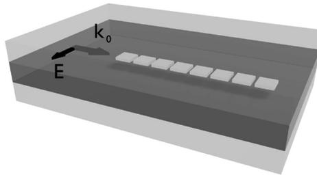
Figure 1: A chain of eight gold particles embedded in a dielectric waveguide and illuminated by a TE-polarized mode.
