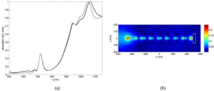
Figure 4: (a) Absorption spectra of the eight-particle chain without (black) and with (gray) chromium block placed 20 nm away from the last particle ; (b) Amplitude of the electric field along the middle of the chain, with the chromium block.
