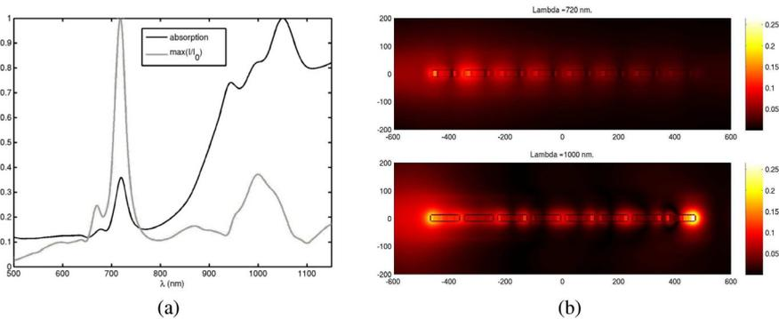
Figure 2: (a) Absorption and electric-field maximal-amplitude spectra, normalized to their maximum ; (b) Distribution of the electric-field amplitude in the plane perpendicular to the middle of the chain, for the two resonances of the maximal-intensity spectrum.
