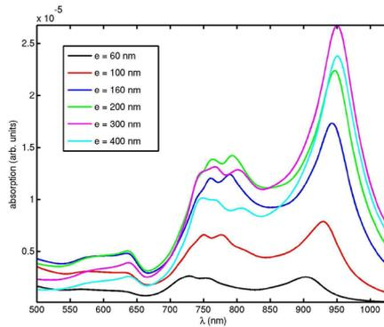
Figure 3: Evolution of the absorption spectra with the thickness of the silica waveguide.
