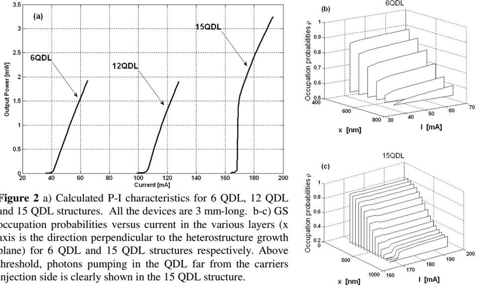
**Figure 2** a) Calculated P-I characteristics for 6 QDL, 12 QDL and 15 QDL structures. All the devices are 3 mm-long. b-c) GS occupation probabilities versus current in the various layers ( $x$  axis is the direction perpendicular to the heterostructure growth plane) for 6 QDL and 15 QDL structures respectively. Above threshold, photons pumping in the QDL far from the carriers injection side is clearly shown in the 15 QDL structure.
