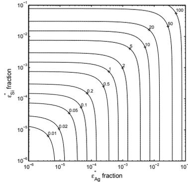
Figure 3: Contour plot of the loss values in dB/μm when the  $\epsilon''$  values of both Ag and Si are varied in fractions of their natural values at room temperature.
