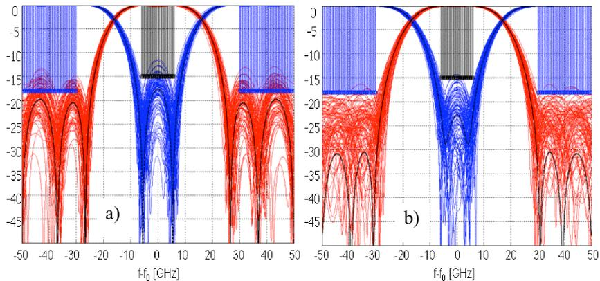
Fig. 2 - Impact of the tolerances on a 7-cascaded Mach-Zehnder before a) and after b) yield optimization.
