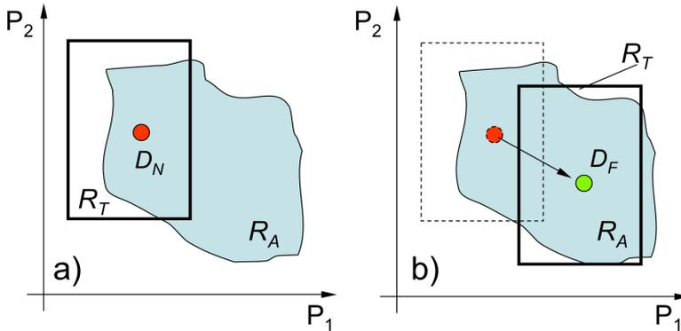
Fig. 1 – Yield maximization and design centering by using information on parameters tolerances.
