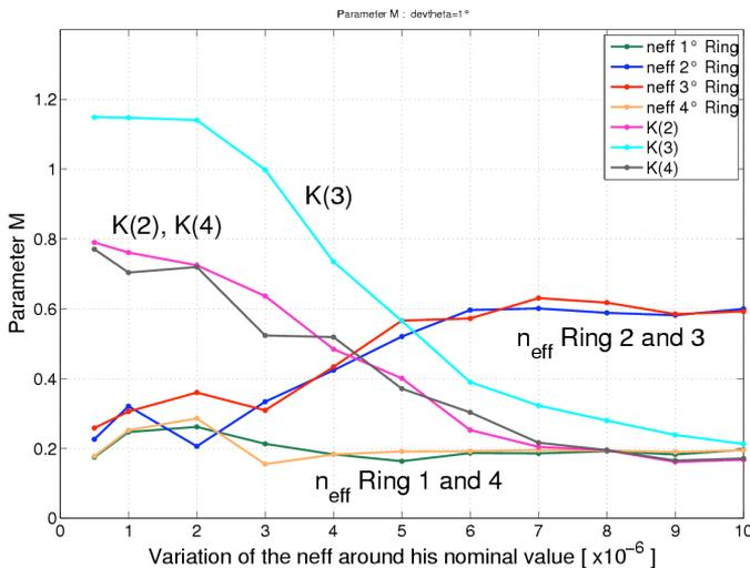
Fig. 3 – 4-cascaded ring filter. Parameter  $M$  of the central couplers and of the refractive index of the rings versus the standard deviation of the refractive index.
