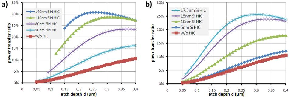
Figure 3: Calculated PTR of a  $1\ \mu\text{m}$  thick polymer waveguide as function of the etch depth  $d$  for a) a SiN ( $n=2$ ) and b) amorphous Si ( $n=3.48$ ) HICs.
