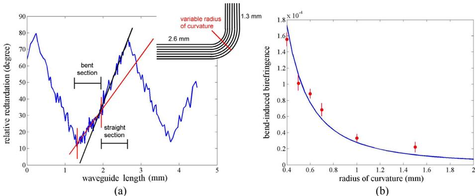
Fig. 2. (a) Measured spatial behaviour of birefringence-induced phase retardation in a waveguide with a bent section of radius  $R=400\mu\text{m}$ . (b) Bend-induced birefringence as a function of the radius of curvature.
