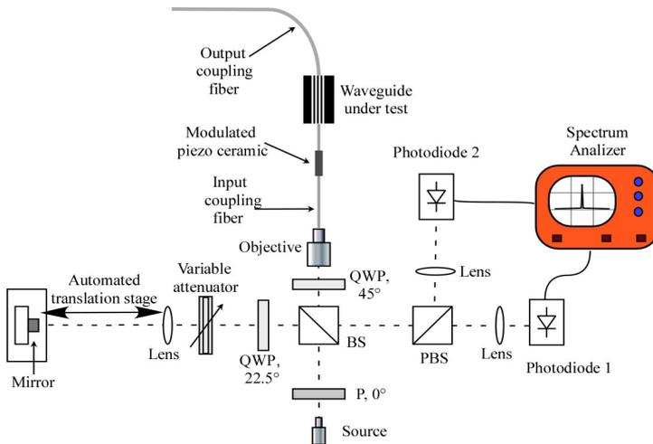
Fig. 1. PS-OLCR experimental set-up. BS=beam splitter; P=polarizer; QWP= $\lambda/4$  waveplate.
