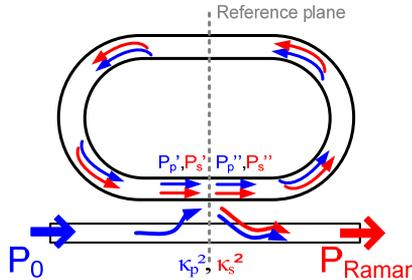
**Fig.1: Schematic view of a racetrack resonator.  $P_0$  represents the initial pump power,  $P_{Raman}$  the output power of the Raman laser at the Stokes wavelength  $\lambda_s$ .  $\kappa_{p/s}^2$  describe the wavelength dependent coupling coefficients between bus waveguide and resonator.**
