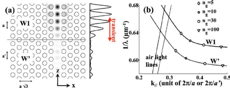
Figure 1: Simulations performed using a Bloch mode Fourier modal method, showing the smooth transition between the injector region and the main crystal (a). Dispersion relations for the W1 and W1' regions are shown on the right (b) [7].
