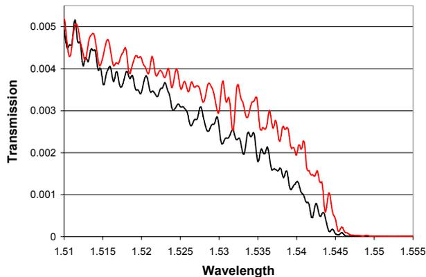
Figure 3: Transmission spectra for a normal W1 (black) and a W1 with 10 period injector regions with a 20 nm period enlargement (red). The nominal lattice constant was 420 nm and the W1 length was 200  $\mu\text{m}$ . The shape of the transmission curves is also influenced by the propagation loss, which is higher in the slow light regime.
