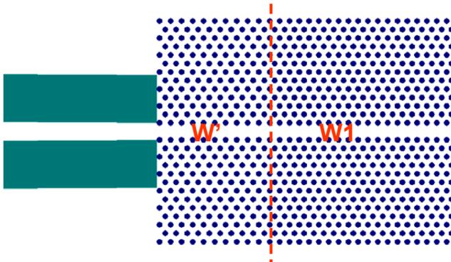
Figure 2: An example of a W1 photonic crystal waveguide with a coupling region (W') between the slow light region (W1) and the access photonic wire. The lattice constant along the direction of the defect is enlarged in the coupler region. For illustrative purposes the enlargement shown here is 50 nm.
