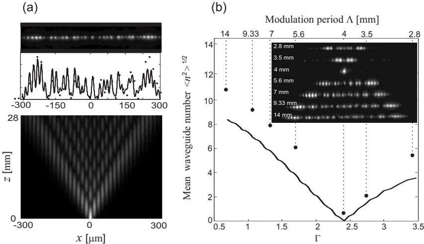
Figure 1: Optical analogue of electronic dynamic localization in an array of sinusoidally-curved waveguides (Ref.[9]). By varying the period  $\Lambda$  of waveguide bending, discrete diffraction in the array [in panel (a)] can be suppressed [see panel (b)].
