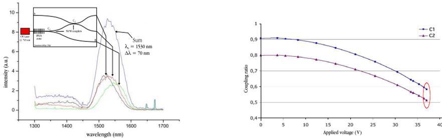
Figure 2: (a) – SPDC from the non-linear waveguide zone, see the text for explanations. (b) – Characterization of the coupling ratios obtained with couplers  $C_1$  and  $C_2$  in both classical (lines) and single photon counting (dots) regimes.
