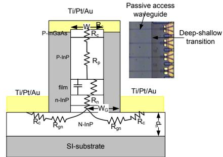
Figure 1: Active-passive butt-joint layer-stack with specifications based on a semi-insulating substrate .
