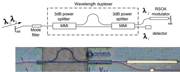
Figure 1: (Up) The layout of the integrated transceiver consisting of a wavelength duplexer, a reflective SOA modulator and a detector. (Below) The fabricated transceiver used for characterization.
