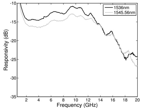
Figure 5: The measured frequency response of the wire bonded photodetector at  $-6$  V when  $P_{in} = -20$  dBm.
