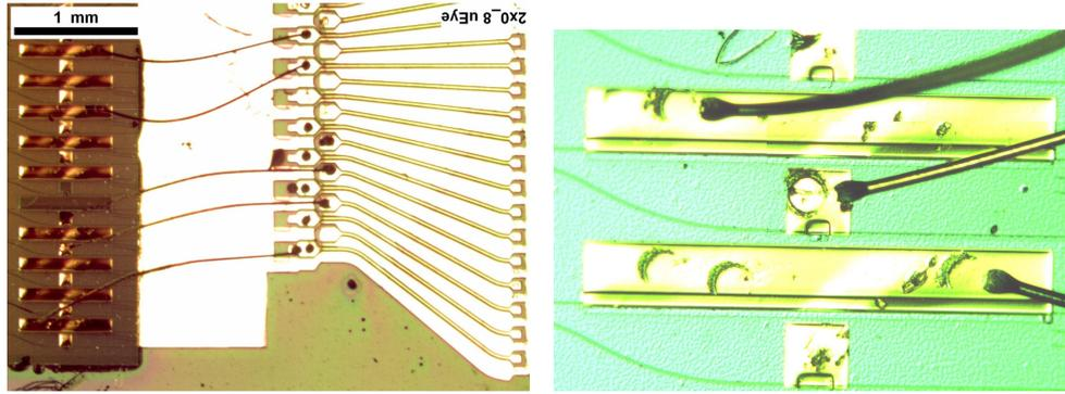
Figure 3: Bonded chip on a AlN RF submount (left) and bonded RSOA and the photodetector (right).
