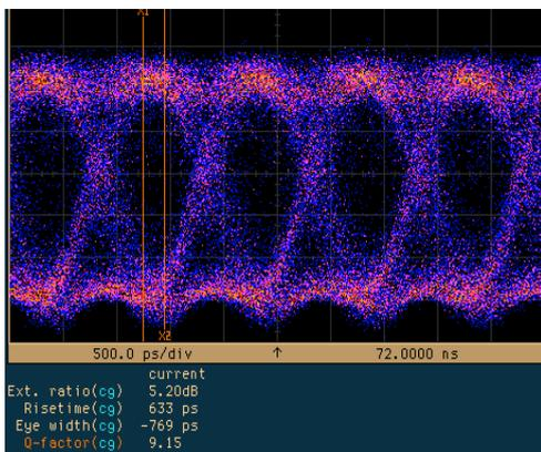
Figure 4: 1 Gbit/s eye diagram at  $\lambda = 1541.9$  nm with input optical power  $P_{in} = -11$  dBm, 80 mA injection current and 0.78 V modulation depth.
