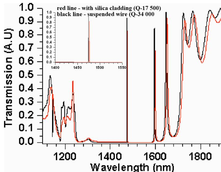
Figure 2: 3D FDTD computed for tapered one-dimensional PhC/PhW micro-cavities embedded in 500 nm photonic wire waveguides with cavity length,  $c \sim 425$  nm for suspended wire (red line) and without removal of the silica buffer lower-cladding layer (black line).
