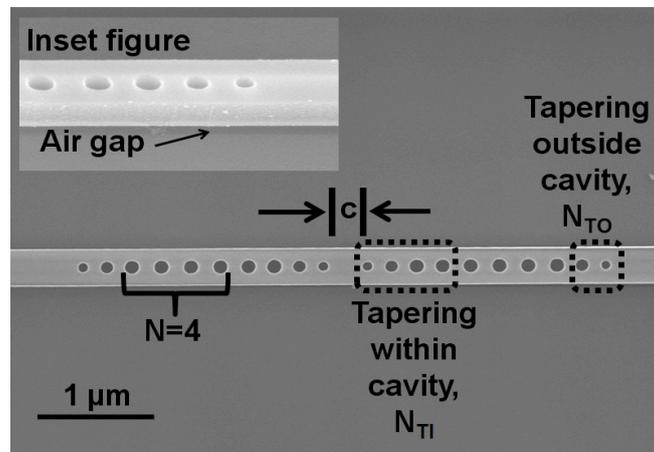
Figure 1: SEM image of an air bridge type of tapered single-row PhC/PhW waveguide with cavity length,  $c$ , four hole tapers within the cavity - and two hole tapers outside the cavity. Inset is a bird's eye view (angle  $\sim 25^\circ$ ) of the suspended PhC/PhW micro-cavities.
