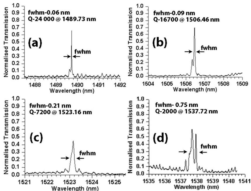
Fig 3: Measurement result for suspended PhC/PhW micro-cavities in a suspended wires with cavity lengths, c (a) 390 nm (b) 415 nm (c) 440 nm (d) 465 nm
