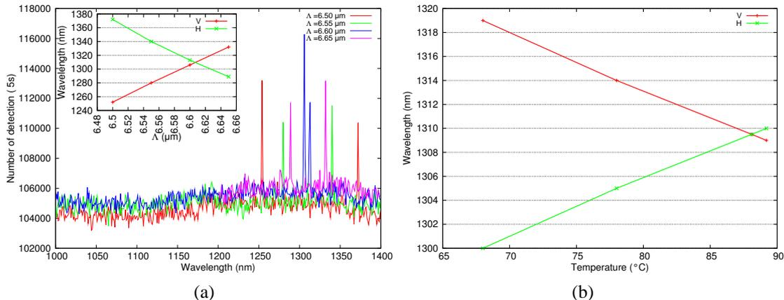
FIG. 2: (a) Fluorescence spectra, obtained in the single photon counting regime, for various poling periods associated with a  $6\ \mu\text{m}$ -wide waveguide heated to  $80^\circ\text{C}$  when pumped at  $655\text{nm}$ . (b) QPM curve as function of the temperature for  $\Lambda = 6.60\ \mu\text{m}$ ; The degeneracy point can be reached by fine tuning of the temperature up to  $88^\circ\text{C}$ .
