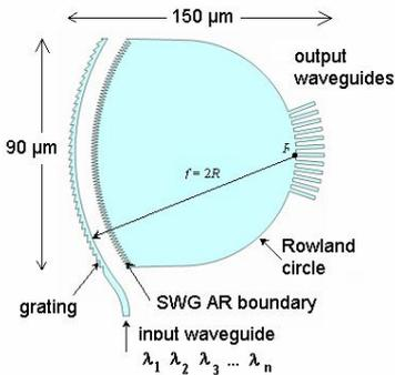
Fig 1: Waveguide grating demultiplexer
