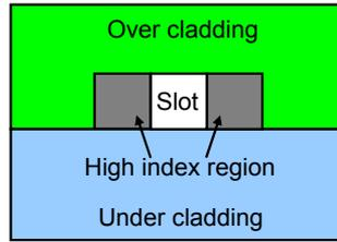
Fig. 1 Cross-sectional schematic structure of a slot waveguide
