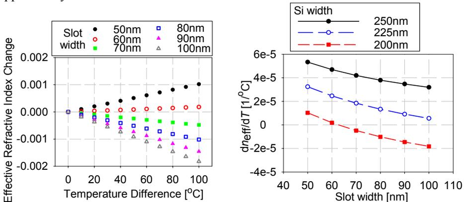
Fig. 2(a) Simulated temperature dependence of effective indices with several slot width
