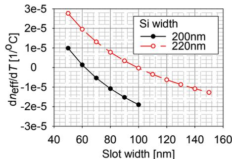
Fig. 3 Temperature insensitivity design with different Si width without changing waveguide heights (250nm)
