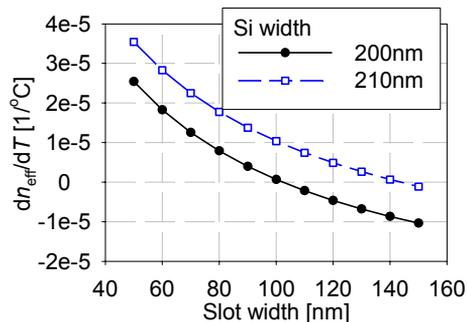
Fig. 5 Effective refractive index slopes of Si slot waveguides with SiO<sub>2</sub> slots, 250nm heights, TE modes
