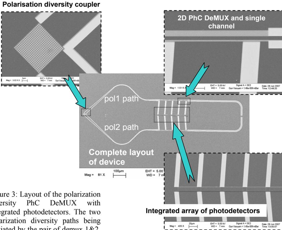
Figure 3: Layout of the polarization diversity PhC DeMUX with integrated photodetectors. The two polarization diversity paths being deviated by the pair of demux 1&2, and recombined in the array of photodiodes, including the 'through' waveguide.
