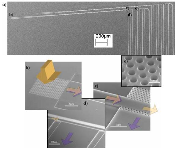
Figure 2: Experimental data from seven-channel demux with cleaved edge. A good separation of 7 optical channels with a spectral resolution of 10 nm nearly suitable for coarse WDM at 20 nm spacing is achieved.
