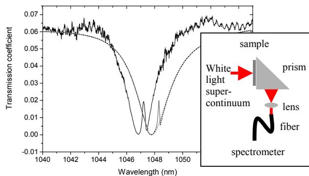
**Fig. 5:** Transmission coefficient of the structure around 1050 nm after suppression of backside reflection (insert). The grey curve is the theoretical transmission coefficient taking into account the measured grating parameters (period of 559.1 nm and depth of 17 nm). The dashed curve is the theoretical spectrum obtained under an incidence angle of  $0.015^\circ$
