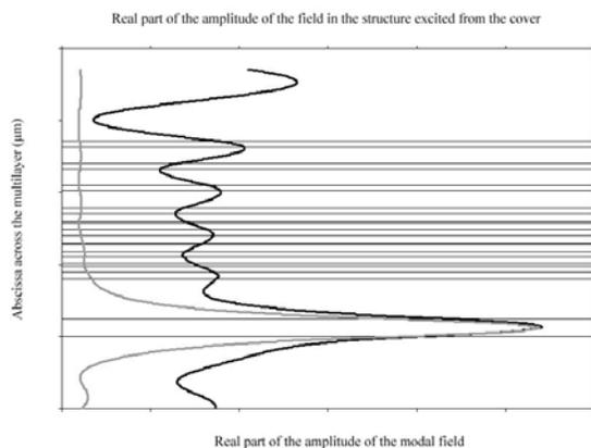
**Fig. 4:** Transverse electric field profile in the multilayer. Grey curve:  $TE_0$  modal field, Black curve: field profile upon excitation from the air side. The horizontal lines show the different layers of the stack.
