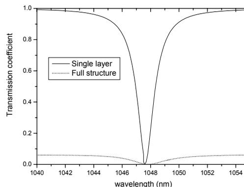
**Fig. 2:** Calculated transmission coefficient of the complete resonant mirror (dotted line) and of the sole waveguide submirror (full line) versus wavelength in the resonance neighbourhood.
