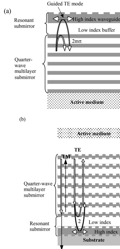
**Fig. 1:** (a) Operation principle of a polarizing mirror integrated to the active medium [2], (b) of a longitudinal mode filter. In both structures light experiences constructive interference between multilayer and resonant submirrors.
