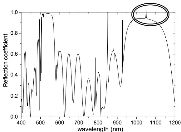
**Fig. 3:** Reflection coefficient of the optimised structure versus wavelength in the visible and IR regions with a peak at 1050 nm.
