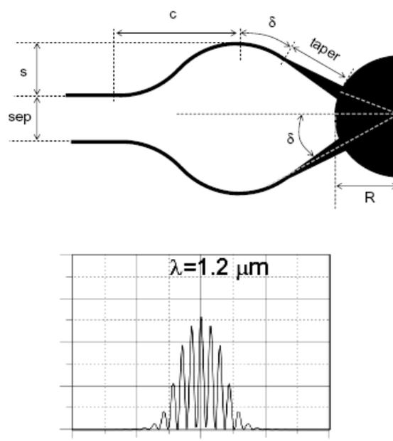
Figure 5 – Schematic representation of a two beam combiner and intensity distribution at the output plane.
