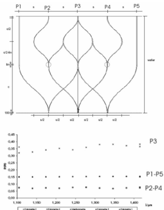
Figure 3 – (a) Schematic layout of a three beam combiner and (b) power output as a function of wavelength.
