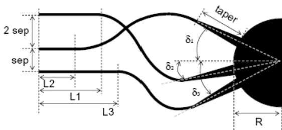
Figure 4 – Schematic representation of a multi-axial beam combiner (in this case,  $\delta_1 > 0, \delta_{2,3} < 0$ ).
