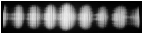
Figure 6 – Experimental intensity pattern at device output imaged in the sensor of a vidicon camera using a 4× microscope objective lens, using a semiconductor laser at 1.3μm. The spatial period is  $\approx 20.5\mu\text{m}$ , in good accordance with the expected value (20.0μm). The vertical lines are an artefact of the image.
