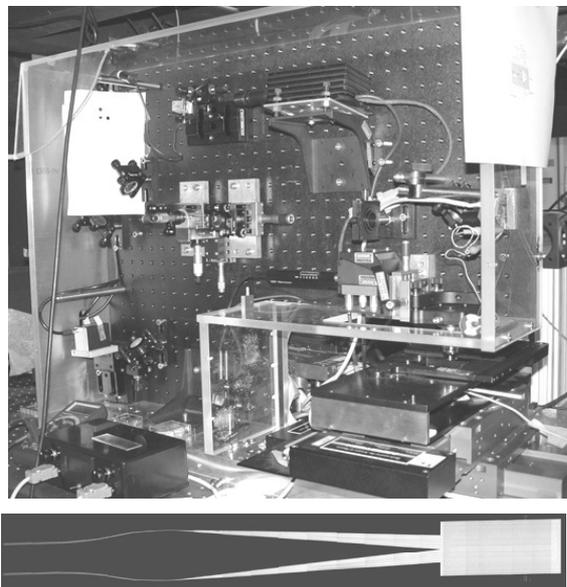
Figure 1 – Photograph of the laser direct writing unit and picture of the multiaxial two beam combiner written in mask photoblanks
