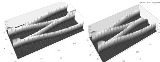
Figure 2 – Field amplitude along the two beam combiner for inputs in phase and  $\pi$  out of phase.
