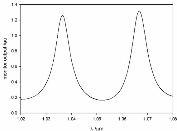
**Fig. 2:** FSR for FW in a z-cut LiNbO<sub>3</sub> regular hexagonal micro-cavity when  $\alpha = 5.973 \mu\text{m}$ .
