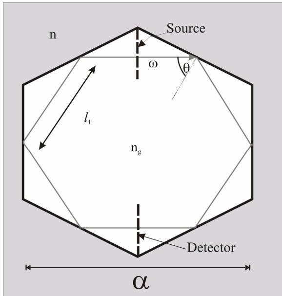
**Fig. 1:** Regular hexagonal optical cavity showing the optical path of the fundamental wave  $\omega$ .  $\alpha$  is the distance between opposite walls and  $l_1$  is the propagation length between sequential reflections.
