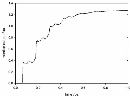
**Fig. 3:** Cavity build-up for FW in a z-cut LiNbO<sub>3</sub> regular hexagonal micro-cavity for  $\lambda_{\omega} = 1.064 \mu\text{m}$ .
