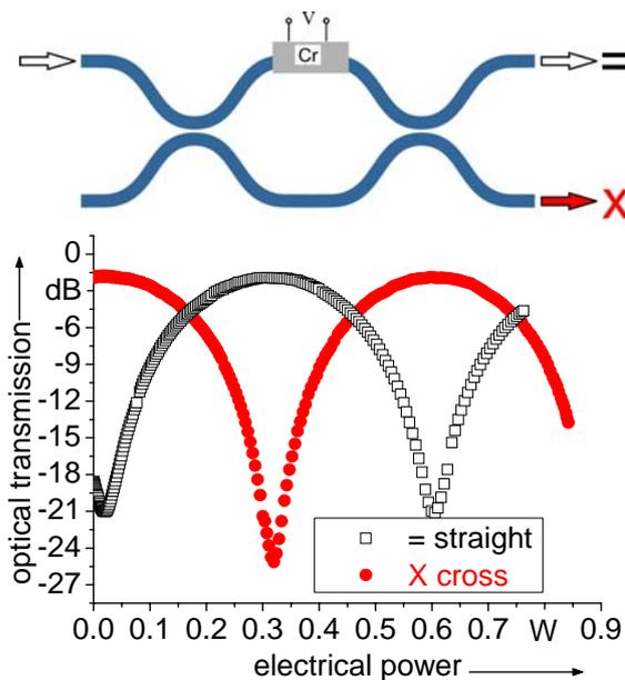
**Fig. 4:** Thermo-optic control of a tunable MZI-coupler
