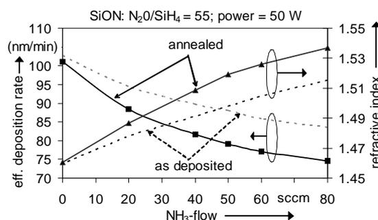
**Fig. 1:** a) Deposition parameters for SiON- and SiO<sub>2</sub>-layers; b) refractive index and deposition rate before and after  $1150^\circ\text{C}$  annealing in dependence on the  $\text{NH}_3$ -flow
