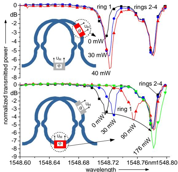
**Fig. 6:** Tuning the phase shifters of one of four ring resonators, which are based on a tunable MZI. The resonance depth is controlled by the MZI-phase. The resonance wavelength is shifted by the thin-film heater in the feedback path.
